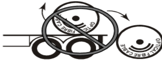
Fig.12. Loading/Unloading of Cable Drums
